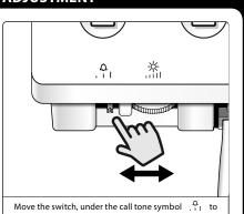
Move the switch, under the call tone symbol  $\begin{bmatrix} \Delta \\ -1 \end{bmatrix}$  to adjust the call tone volume level. Move to the left for a low call tone level, to the centre for a medium call tone level and to the right for a high call tone level.
