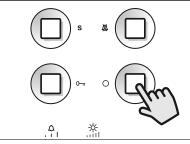
Pick up the handset and then push the camera recall button  $\bigcirc$  as many times as the ID value of the door panel (e.g. if recalling the picture from door ID 2, press this button twice, for door ID 3 press this button 3 times etc.). The videophone display will show the picture from the camera on the relevant outdoor station recalled.
